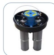
The SP Option is the best automatic filter cleaning system which uses compressed air at 6 bars to clean the cartridges. Thanks to its big surface and very high efficiency, it is possible to work also with huge quantities of fine dust. The filters are aluminated and antistatic, with BIA-M class filtration (EN 60335-2-69). The filter cleaning works when the vacuum cleaner is running.
