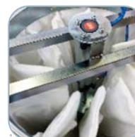
The PSC system is a semiautomatic filter shaker. Inside the filter chamber there is a pneumatic piston which shakes the filter each time the operator pushes the activation button. As an option it is possible to install a PLC to have a complete automatic cycle.
