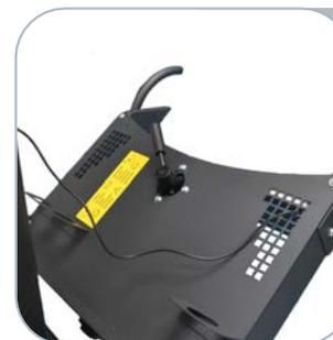
The discharge system is generated by a dedicated system that uses the exhaust air from the turbine. There is an ergonomic leverage that permits to pass from vacuum stage to discharge just in one second. Using the exhaust air the discharge operation is guaranteed also if there are some debris in the liquid.
