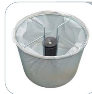
The collected liquid can be filtered through a nylon filter with an efficiency of 150 micron. Thanks to this, it is possible to separate also small debris from the oil and recover the lubricants for reuse. The filter can be washed and reused easily. It is also possible to use a disposal filter with an efficiency of 100 micron.
