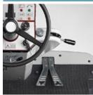
The MACH 5 has a powerful traction system and a top speed of 9 Km/h, this is controlled by a double pedal (forward and reverse directions).
