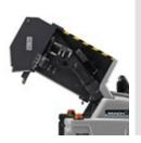
The debris container has a multilevel high dump and is fitted with a hydraulically controlled door. The hopper is fitted in the rear part of the machine and has a 150 L capacity, it can be hydraulically raised to a maximum height of 1350 mm.
